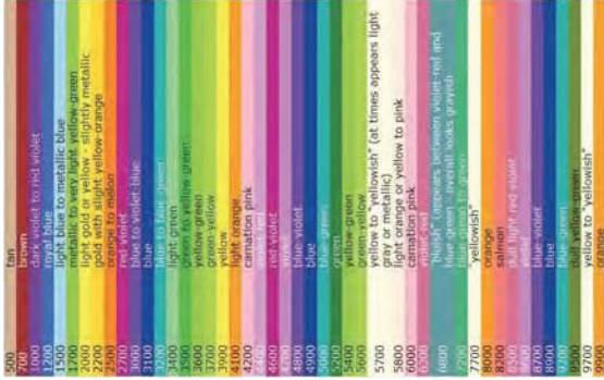
Oxidation Thickness Color Chart
